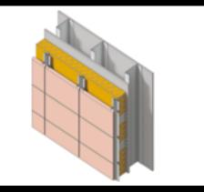
In line with the Building Control Alliance Technical note 18; 'use of Combustible Cladding Materials on residential buildings paragraph 12.7 of AD B2' - use materials of limited combustibility throughout the cladding system.
